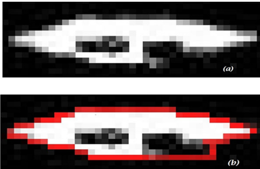
Figure 6 Perimeter and area feature extraction. (a) Extract Perimeter. (b) Area extraction.
